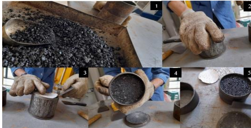
Figure 3. Preparation of the asphalt mixture with RTR-MBs, ELBA ltd laboratory
