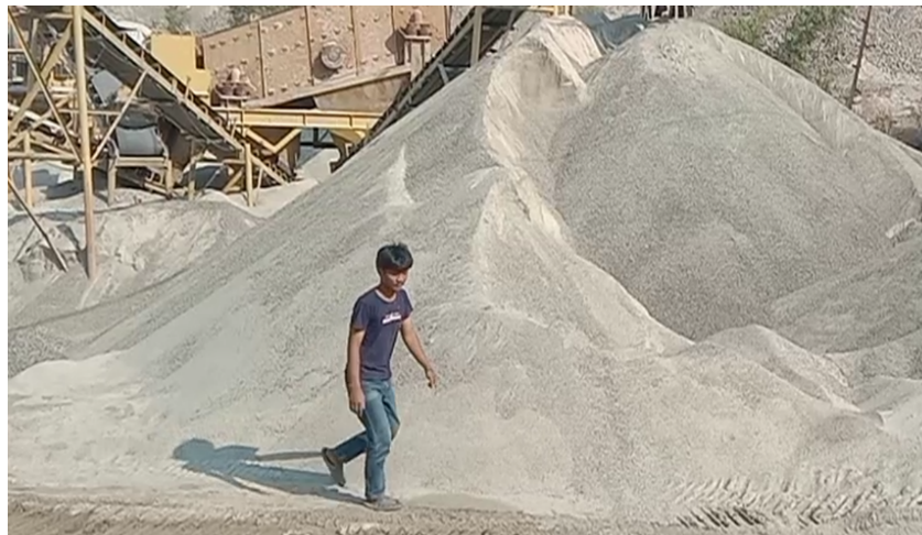
Figure 1. Nickel Slag Pile
