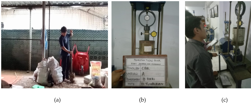
Figure 4. (a) Compaction of CBR samples; (b) and (c) Unsoaked CBR Testing
