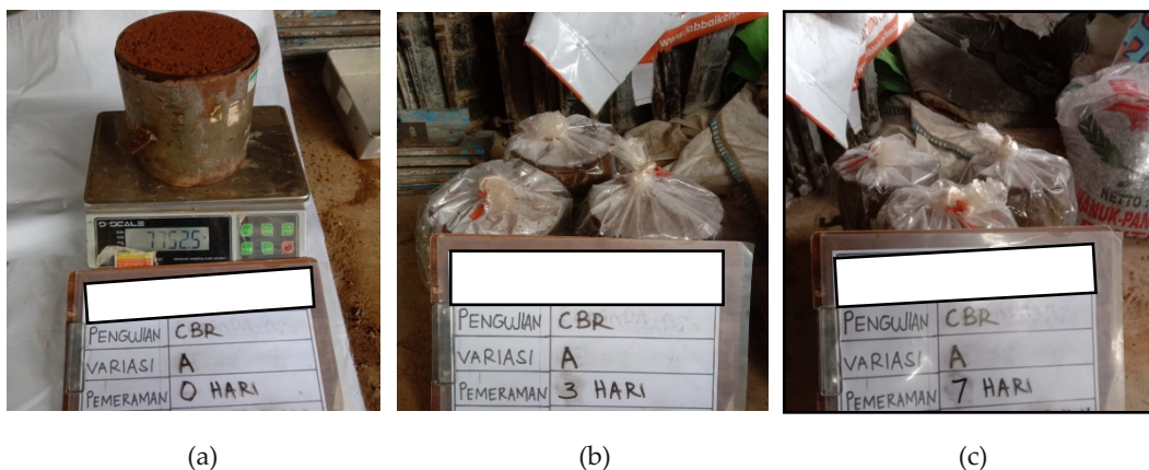
Figure 3. (a)-CBR Test Sample Variation A, curing period 0 days, (b)-CBR Test Sample Variation A, curing period three days, (c)-CBR Test Sample Variation A, curing period seven days.
