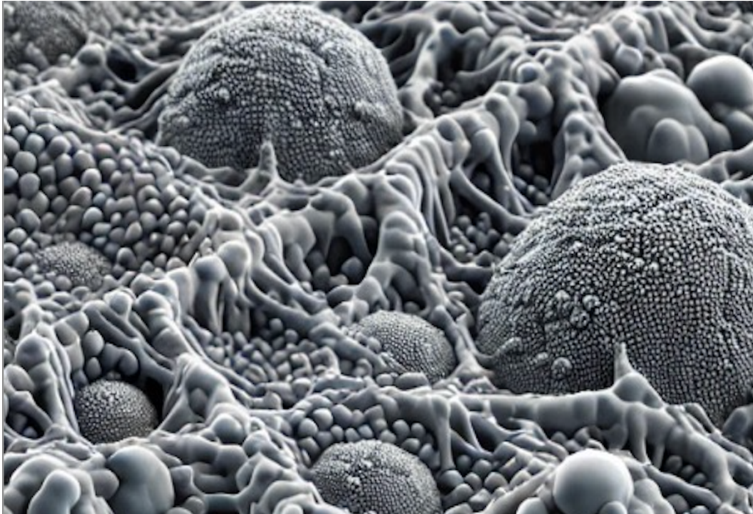
Figure 7. SEM analysis for the effects of sintering at 1000°C on the Ti/SiC composite with a volume fraction of 70% titanium and 30% silicon carbide, inset at 2500x.
