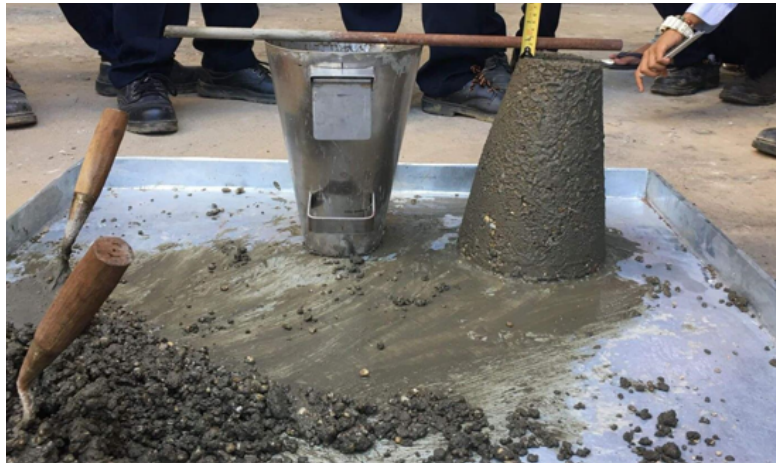
Figure 9. Slump test measured.
