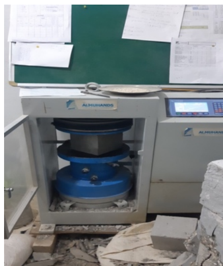
Figure 10. Configuration of a compressive strength test.
