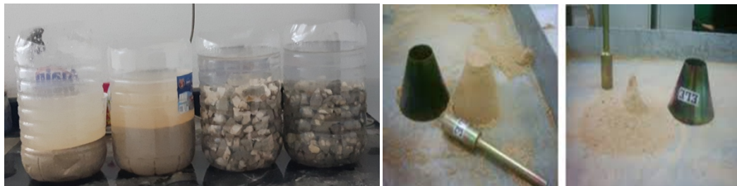
Figure 5. Determine specific gravity for coarse and fin aggregate.
