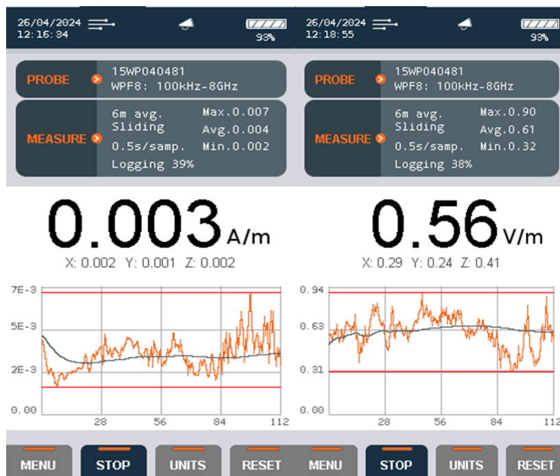
Figure 4. Sequential measurement of field strength E (V/m) and H(A/m).
