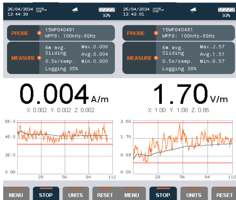
Figure 8. Sequential measurement of field strength E (V/m) and H(A/m).
