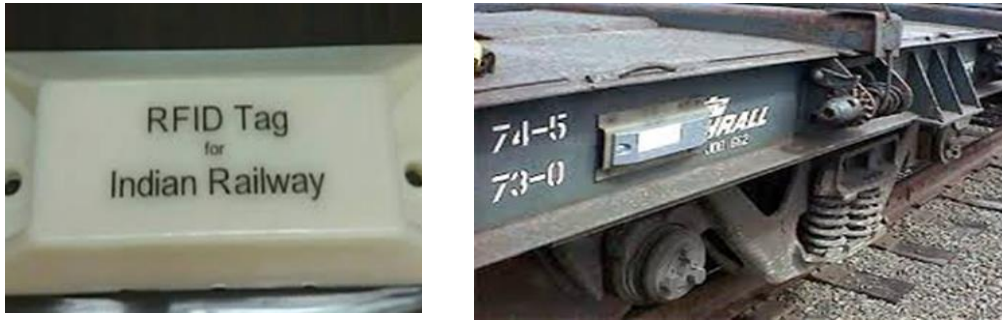
Figure 2. RFID Tag used in IR
