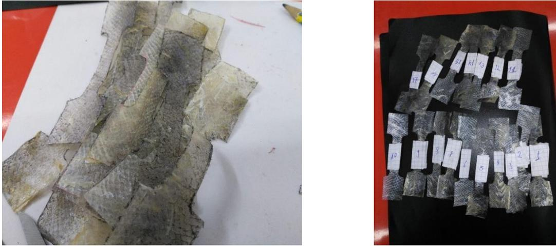
Figure 2. Shape of the fish test pieces for tensile testing
