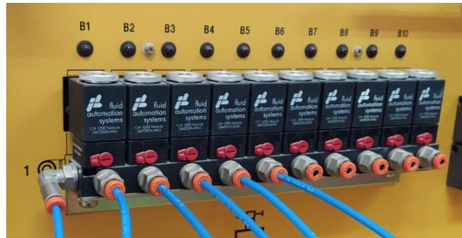
Figure 9. Electro pneumatic valves for stepper motor control
