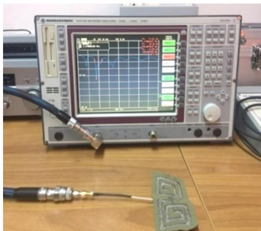
Figure 6. Measurements of the proposed antenna using a Rohde & Schwartz ZVRE Vector Network Analyzer
