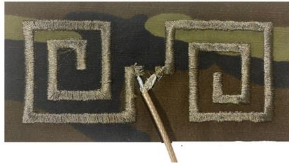
Figure 5. The implemented meander textile presenting the connected 50-ohm coaxial cable
