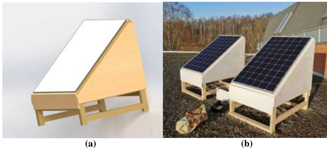
Figure 1. (a) CAD drawing of the test-system. (b) Actual test-systems; S1 at right and S2 at left. (Photo by Jørgen P. Aubell).
