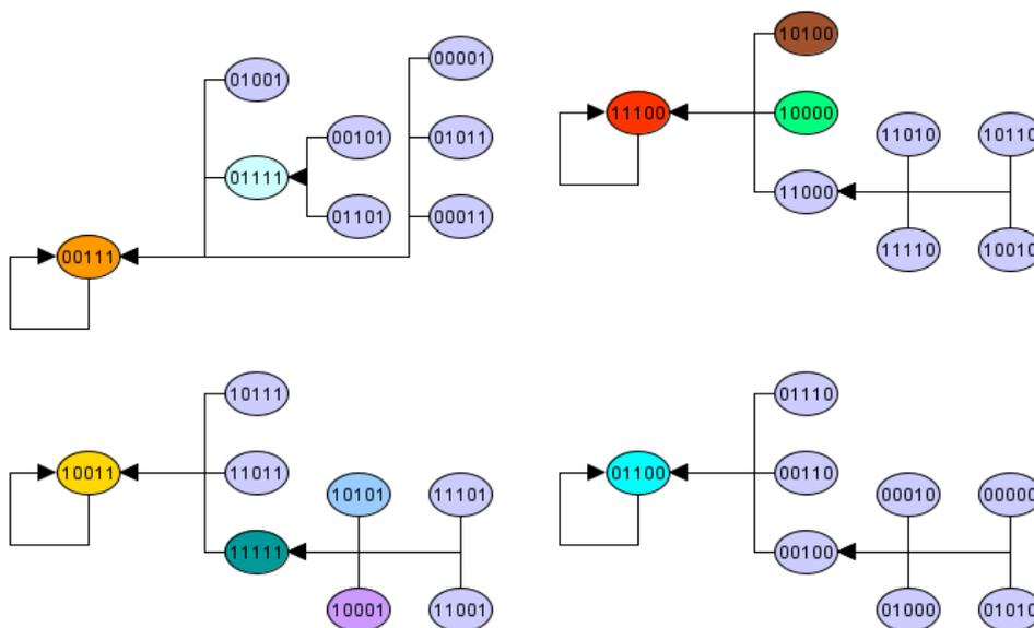
Figure 3. State transition graph created by the simulation of the second Boolean model. Four attractor basins meaning that there are four fixed points which represent four possible stable states:  $\{(00111), (11100), (10011), \text{ and } (01100)\}$ .
