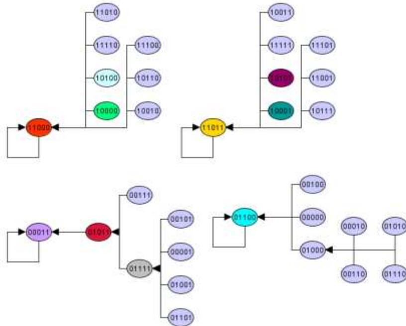
Figure 2. State transition graph created by the simulation of the first Boolean model. Four attractor basins meaning that there are four fixed points which represent four possible stable states:  $\{(11000), (11011), (00011), \text{ and } (01100)\}$ .
