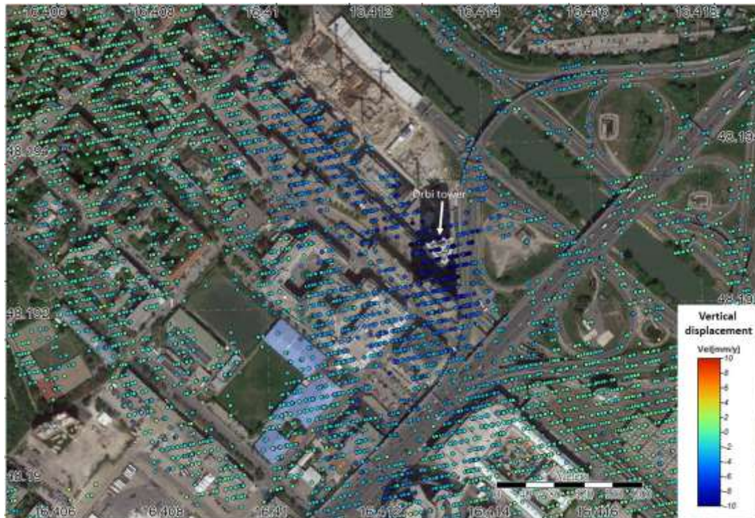
Figure 8. The PSI results at the area of the recently constructed Orbi tower, Vienna. Note the negative displacement rates (shown by light blue to dark blue circles) at the Orbi tower and in the surrounding area. The background is an image of April 5, 2019 from Google Earth™.
