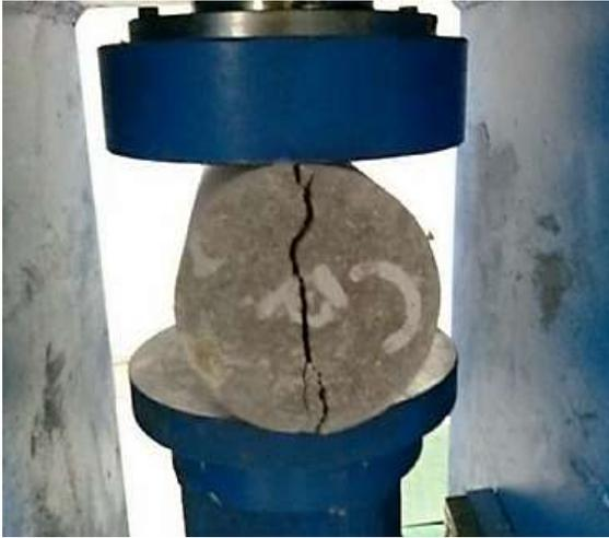
Figure 4. Split tensile strength test setup
