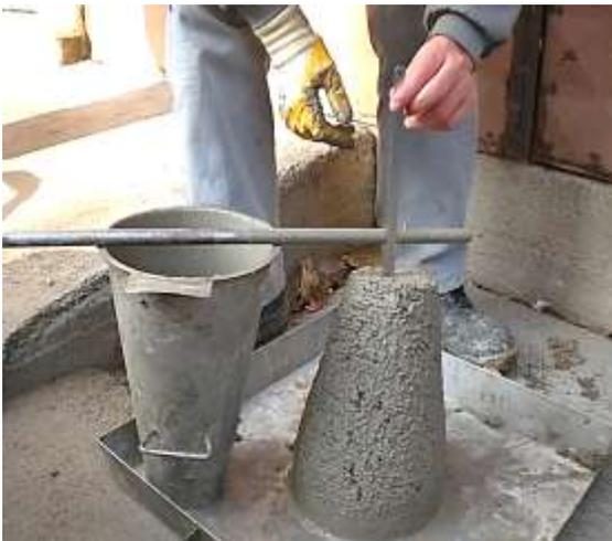
Figure 2. Slump cone test setup
