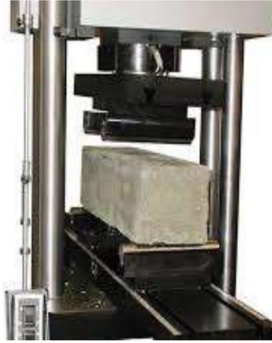
Figure 5. Flexural strength test setup
