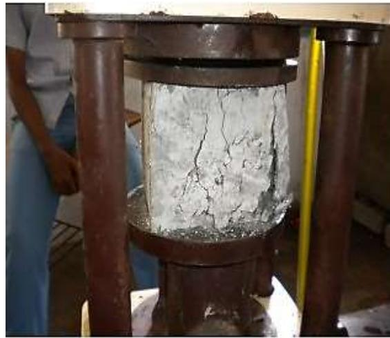
Figure 3. Compressive strength test setup
