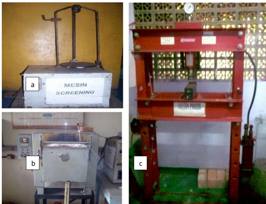
Figure 1. Equipment device of self-propagating high-temperature synthesis (SHS) a) Screening Machine (Sifting) b) Muffle Furnace for SHS c) Press machine to compact sample
