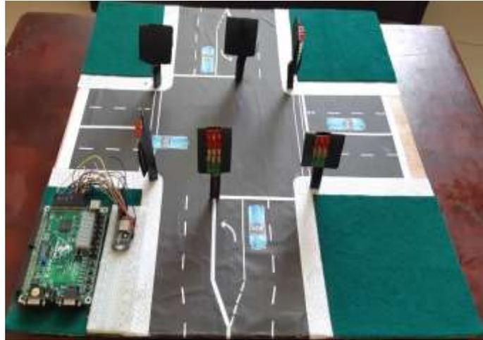
Figure 9. The Complete prototype of the Intelligent Traffic Controller with Remote Control Mode
