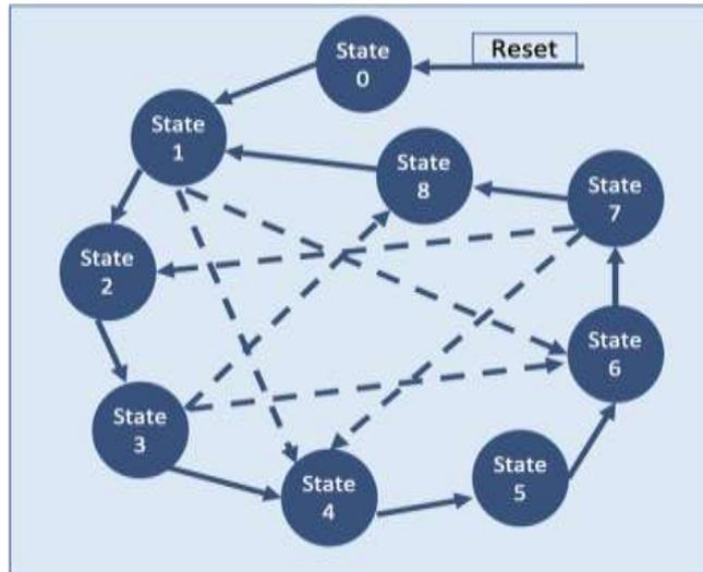
Figure 5. State transition diagram for the Remote Control mode
