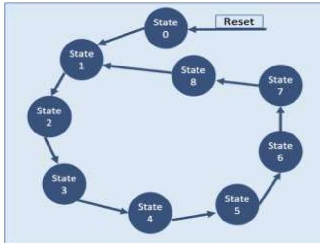
Figure 6. State transition diagram for the Fixed-Time mode
