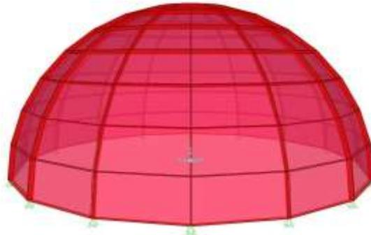
Figure 2. Dome designed without rib beams
