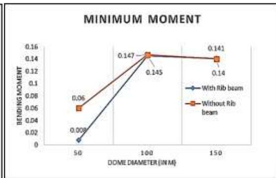
Figure 20. Min. moment vs dome diameter
