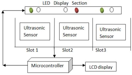
Figure 1. Basic block diagram for parking system
