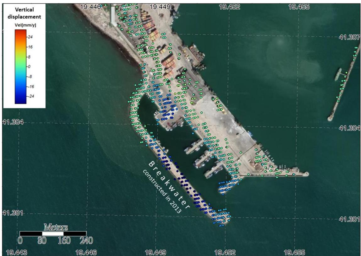
Figure 9. The PSI results of the Sentinel-1 SAR images at the new fishing port of Durrës constructed in 2013. The displacement rates are shown in mm/year.
