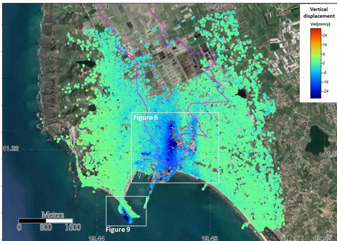
Figure 5. PSI analysis results of the of Sentinel-1 SAR images for the time period January 2017 – December 2018 of the study area, city of Durrës, Albania. The ground displacement rates are shown in mm/year. The results indicate considerable subsidence zones in the southern part of the reclaimed lands of former Durrës marsh. The contour of the former marsh digitized from the Corona satellite image of Figure 1a is plotted onto the map for reference (magenta color line).
