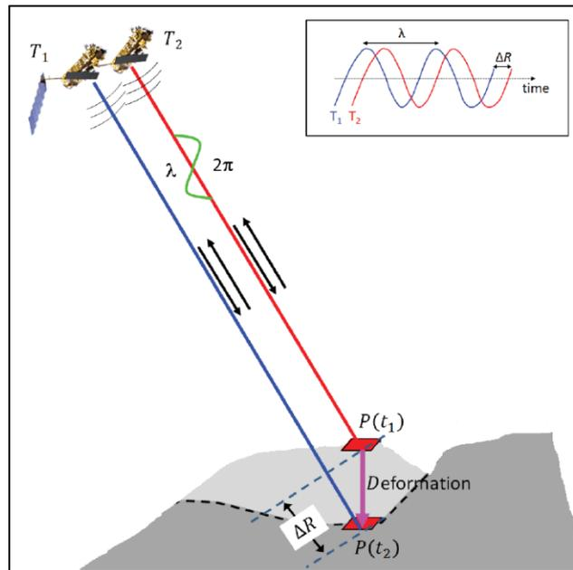
Figure 3. Schematic representation of the DInSAR basic concept. The phase difference of two radar measurements  $T_1$  and  $T_2$  of a ground target  $P$ , recorded at time  $t_1$  and  $t_2$ , due to a subsidence occurring within this time period at the ground target from position  $P(t_1)$  to position  $P(t_2)$  (modified from [17]).
