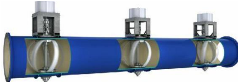
Figure 2. Scheme of hydropower in a pipe
