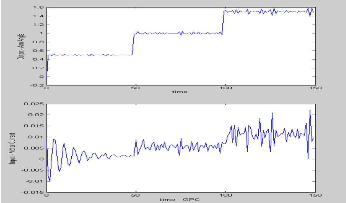
Figure 10. GPC controller with sensor errors (a) Output and (b) Input
