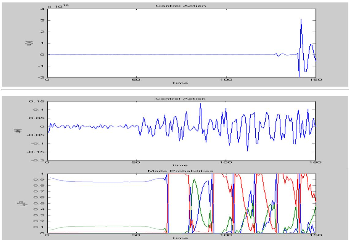
Figure 12. IMM-based GPC failure with very low magnitude of input signal
