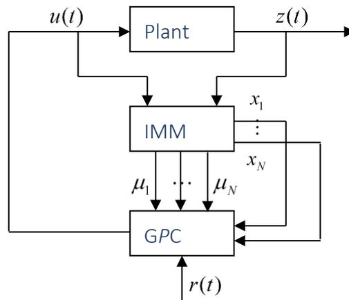
Figure 8. Diagram of IMM based GPC controller
