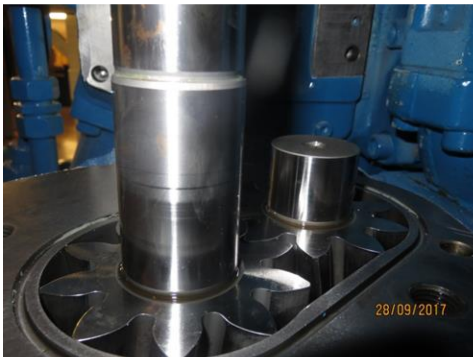
Figure 2.2 pump gears have 10 teeth
