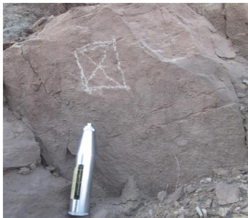
Figure 4: Schmidt hammer used for Rock mechanical strength
