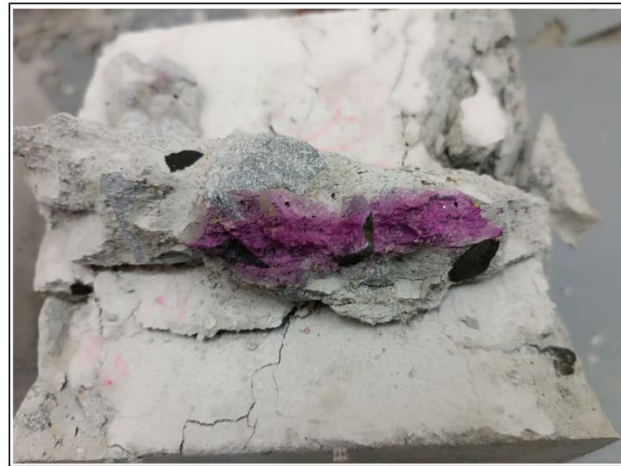
Figure 5. Carbonation Test Sample
