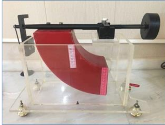
Figure 4. Fabricated hydrostatic position apparatus according to [45]
