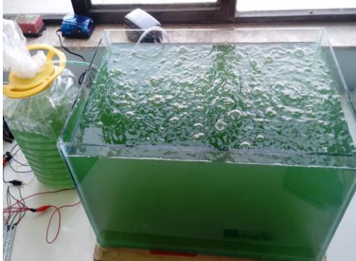
Fig. 4. Lab scale Spirulina photo-bioreactor
